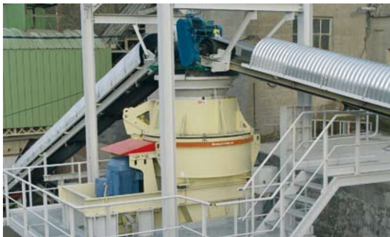
Barmac B7150 vertical shaft impact crusher at a stationary installation in Belgium.
